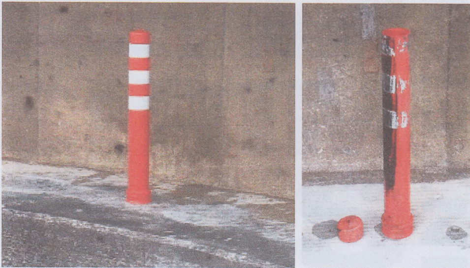
Photo 6 and 7: Photograph before and after. The top of pole cone with extrusion pipe was broken at 588 impacts.
