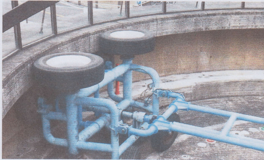
Photo 3: Test condition – Pole cone during impact testing
